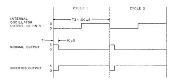
Fig. 2. Pulse generator timing diagram. This shows a pulse train which has a 10-μs pulse width and a 100-μs repetition rate. The duty cycle is equal to 10 μs divided by 100 μs times one hundred percent, which equals 10 percent.
